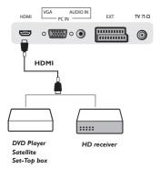
HDMI input compliance with 480i/p, 576i/p, 720p, 1080i/p signal handling capability.
